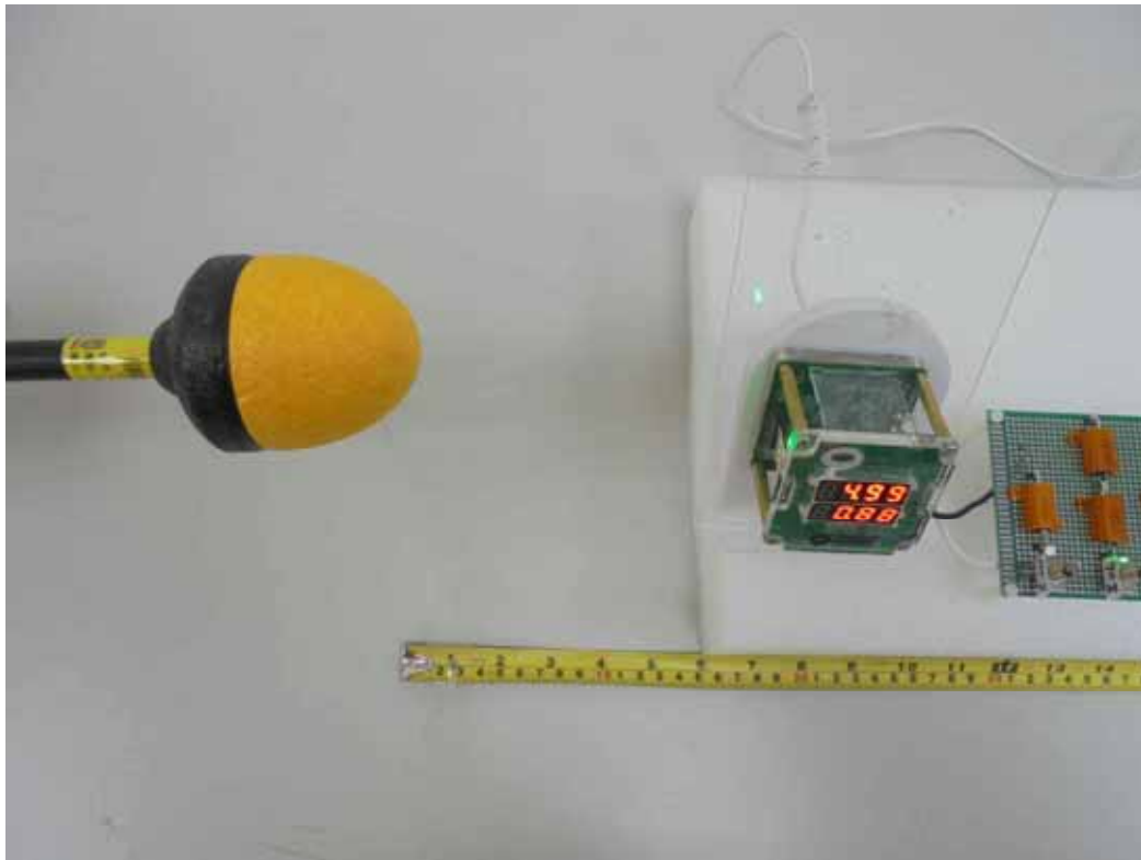
E-Field (Charging Mode with Load with 3mm airgap - Left)
