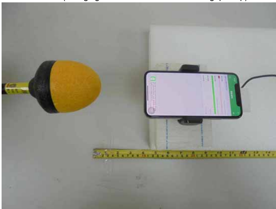
E-Field (Charging Mode with iPhone with 3mm gap - Top)
