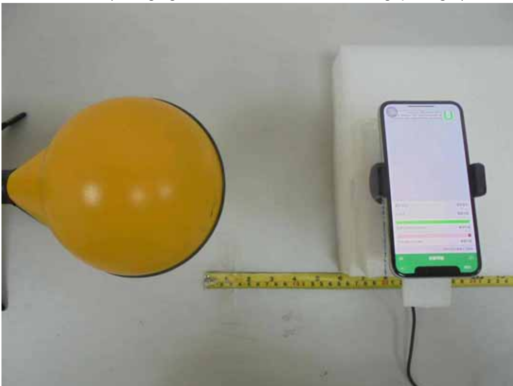
H-Field (Charging Mode with iPhone with 3mm gap - Right)
