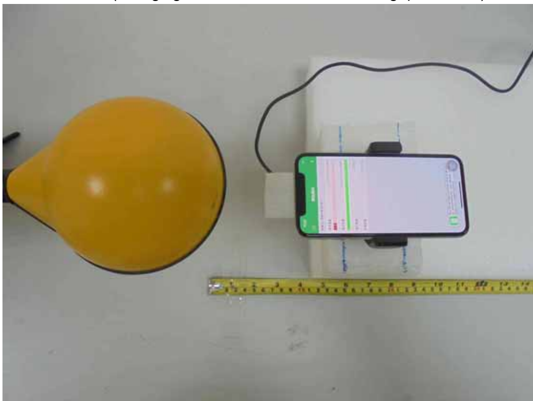
H-Field (Charging Mode with iPhone with 3mm gap - Bottom)
