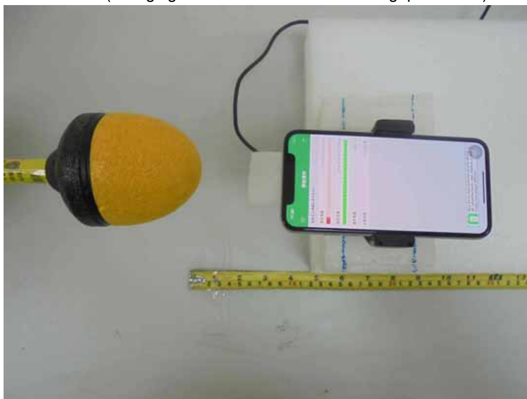
E-Field (Charging Mode with iPhone with 3mm gap - Bottom)
