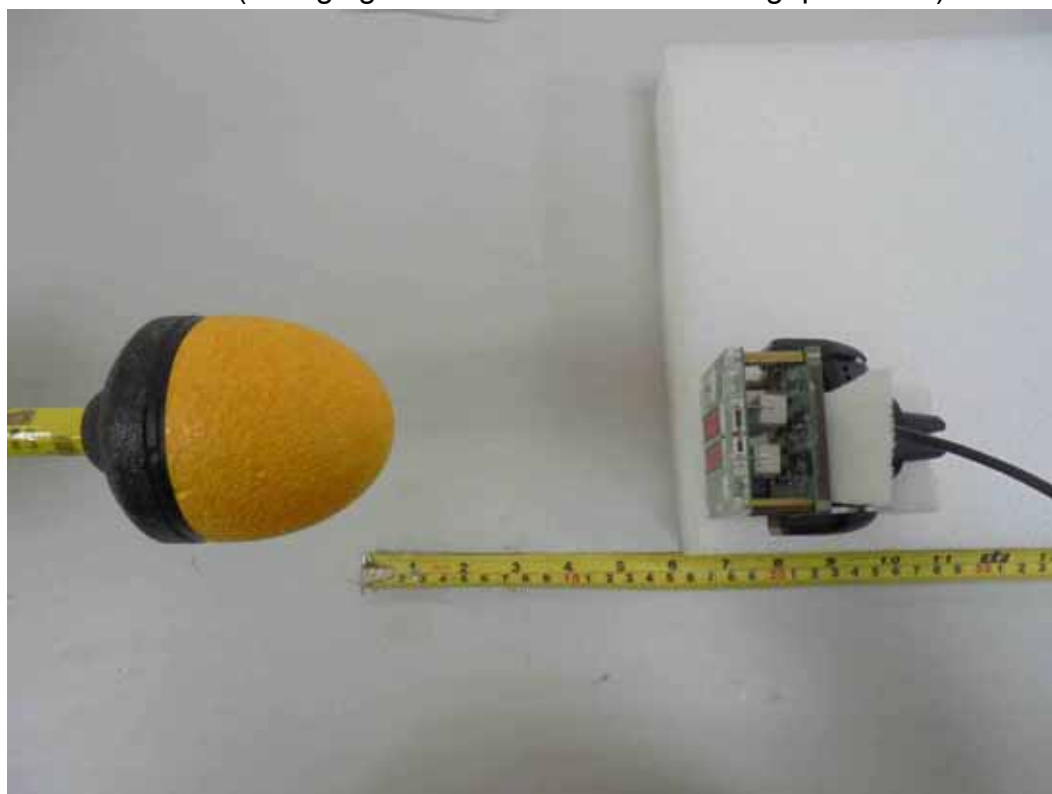
E-Field (Charging Mode with Load with 3mm gap - Z-axis)
