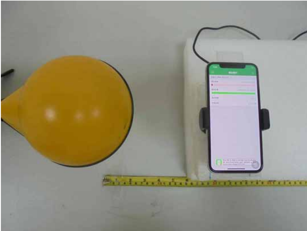
H-Field (Charging Mode with iPhone with 3mm gap - Left)
