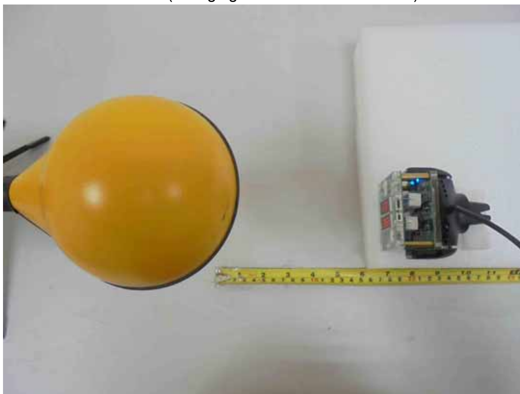
H-Field (Charging Mode with Load - Z-axis)
