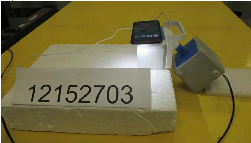
S4, RF EXPOSURE SETUP PHOTO
