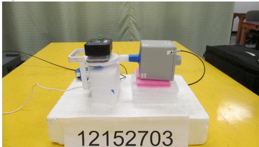
S2, RF EXPOSURE SETUP PHOTO
