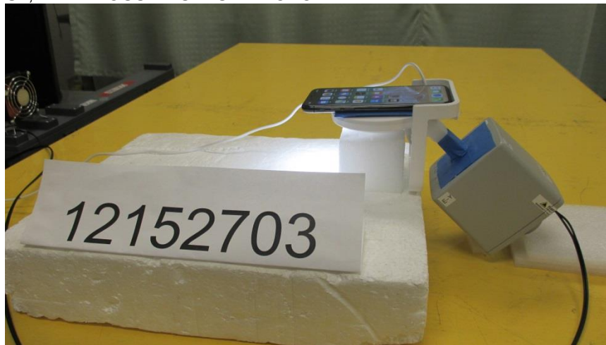
S4, RF EXPOSURE SETUP PHOTO
