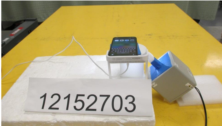
S3, RF EXPOSURE SETUP PHOTO
