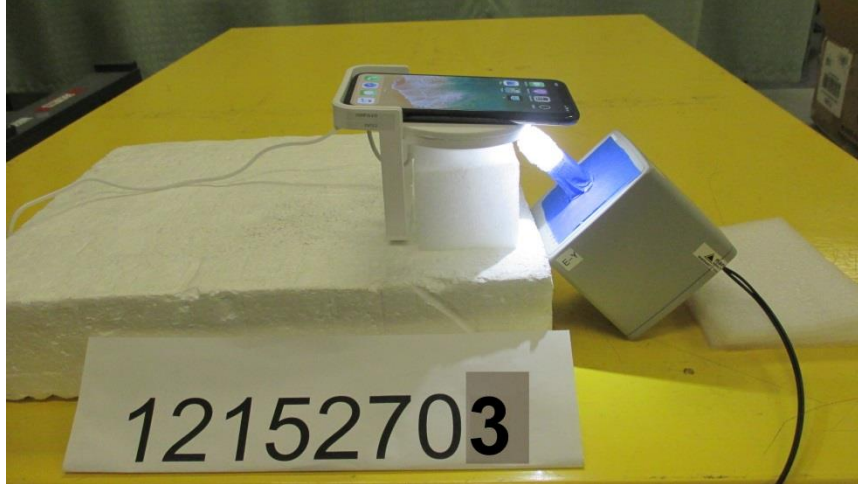
S2, RF EXPOSURE SETUP PHOTO
