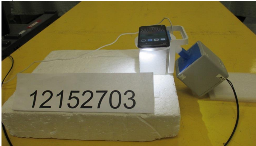
S4, RF EXPOSURE SETUP PHOTO
