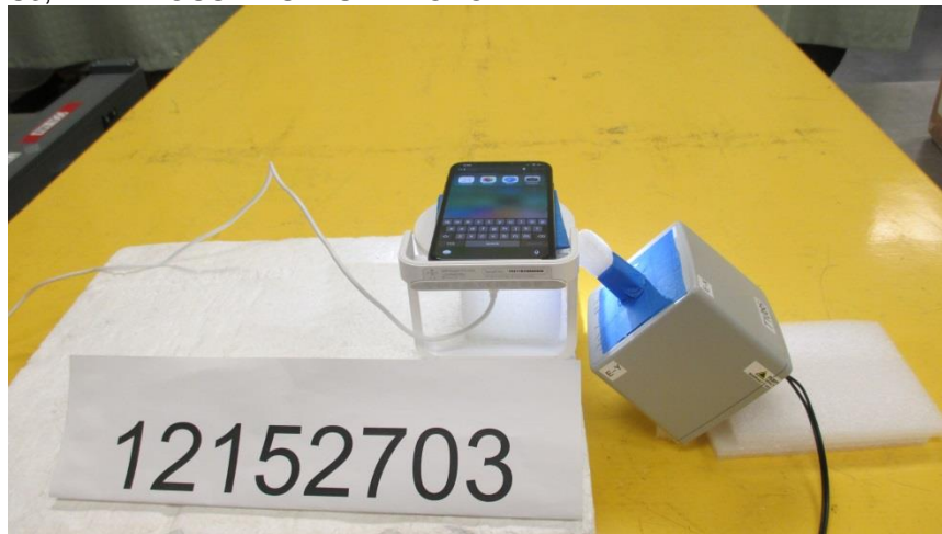
S3, RF EXPOSURE SETUP PHOTO
