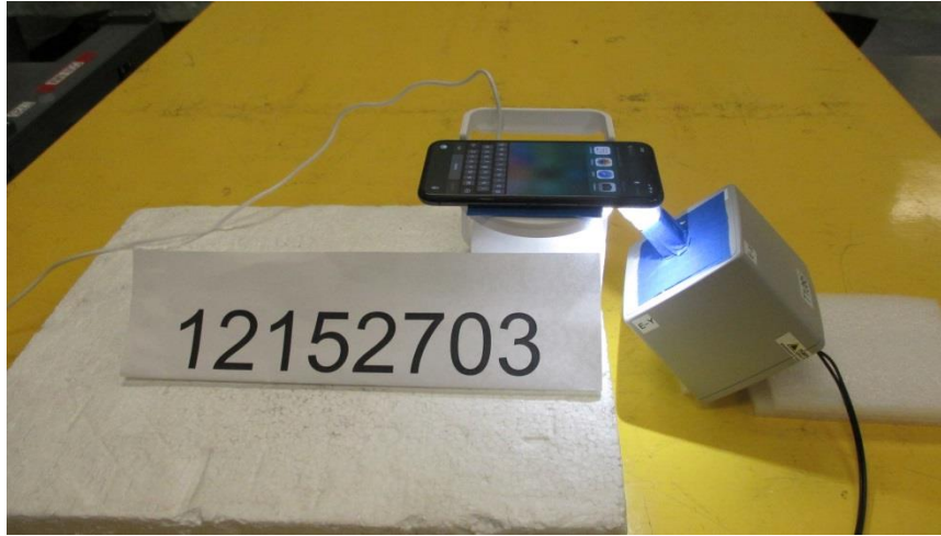
S1, RF EXPOSURE SETUP PHOTO
