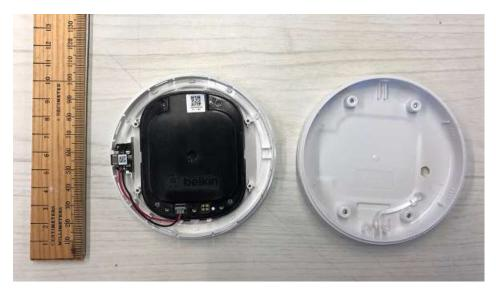
PCB Backside with shield
