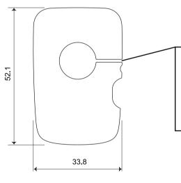
This 1mm wide cut line allows the label to be assembled after the base is installed.
