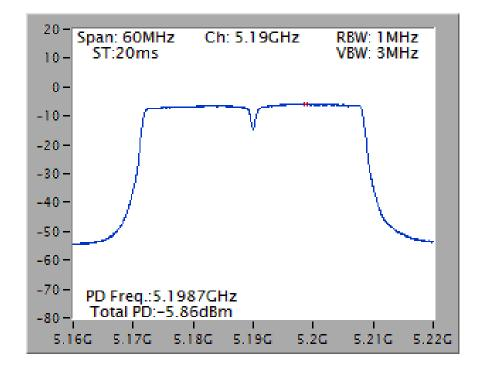
Power Density Plot on Configuration IEEE 802.11n MCS0 HT40 / Chain 1 + Chain 2 / 5190 MHz
