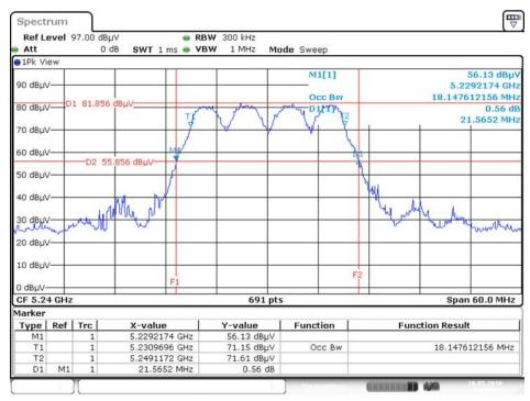
26dB Bandwidth and 99% Occupied Bandwidth Plot on Configuration IEEE 802.11n MCS0 HT20 / Chain 1 + Chain 2 / 5240 MHz
