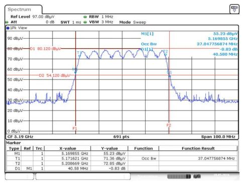
26dB Bandwidth and 99% Occupied Bandwidth Plot on Configuration IEEE 802.11n MCS0 HT40 / Chain 1 + Chain 2 / 5190 MHz
