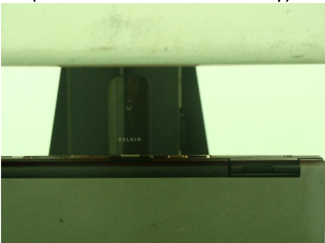
Direct Laptop Plug-in for USB Tip Mode (USB Tip with Phantom 5 mm Gap)
