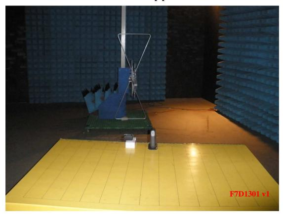
**Photo 2: Radiated Emission Test set-up photo**
