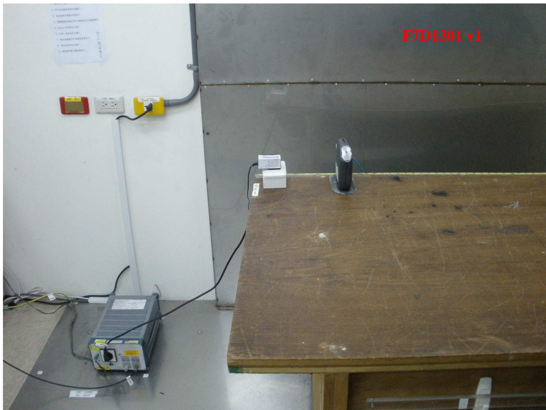
Photo 1: Conducted Emission Test Set-up photo
