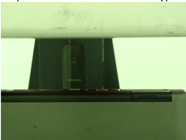
Direct Laptop Plug-in for Tip Mode (Tip Mode with Phantom 0.5 cm Gap)
