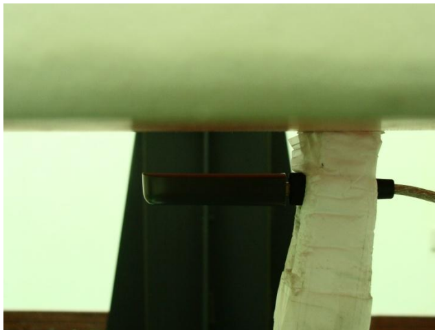
USB Cable Plug-in for USB Configuration 2 (for Back Off SAR) (Horizontal Down with Phantom 1.5 cm Gap)
