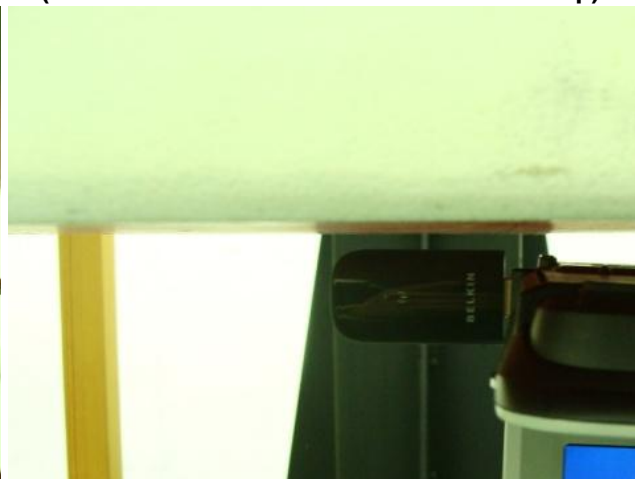
Direct Laptop Plug-in USB Configuration 4 (Vertical Back with Phantom 0.5 cm Gap)
