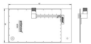
The testboard is designed for evaluation purposes for Rufa 2.4 GHz SMD antenna. The card has the same size as a typical PCMCIA card and is fitted with an SMA connector.
