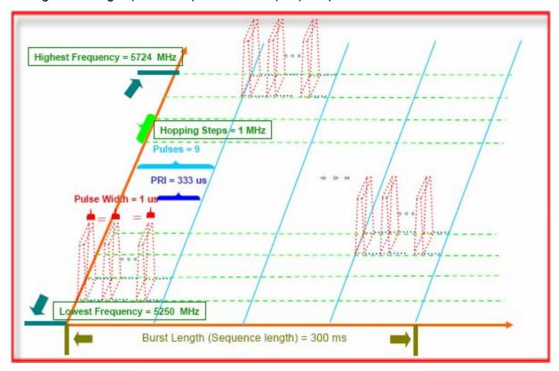
FCC Radar Types (6) System Diagram
