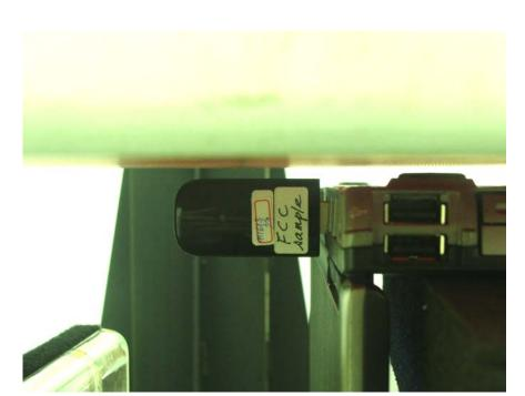
USB Configuration 3 under 5 mm Separation (USB Vertical Front)
