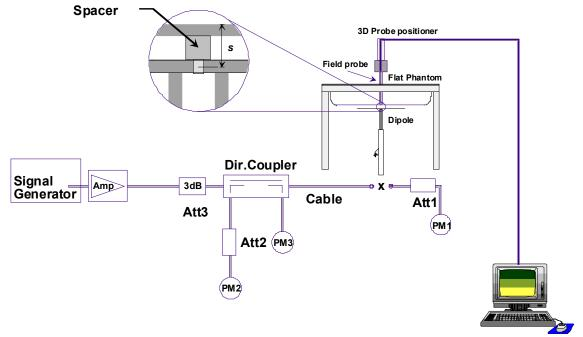
Fig. 8.1 System Setup for System Evaluation
