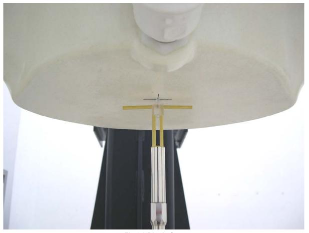
Fig 8.2 Dipole Setup
