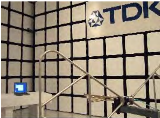
Test Configuration 2. 30 MHz to 960 MHz
