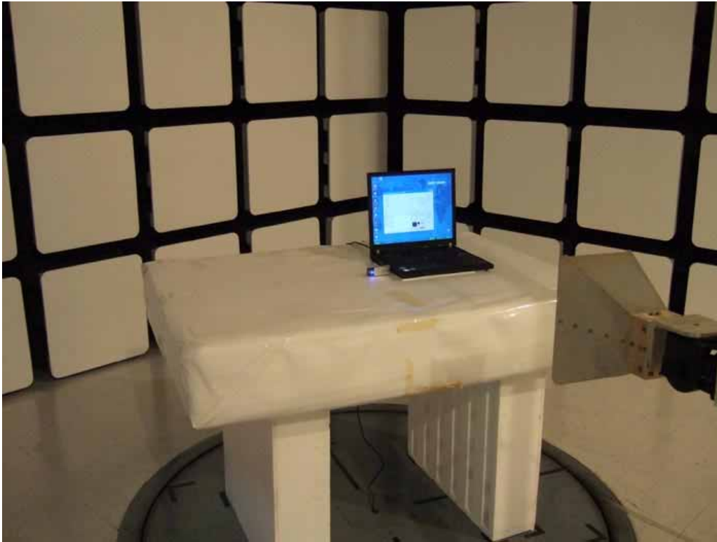
Test Configuration 2: 30 MHz to 960 MHz
