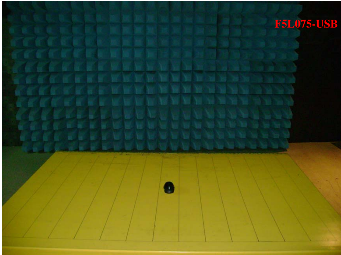
Photo 2: Radiated Emission Test set-up photo
