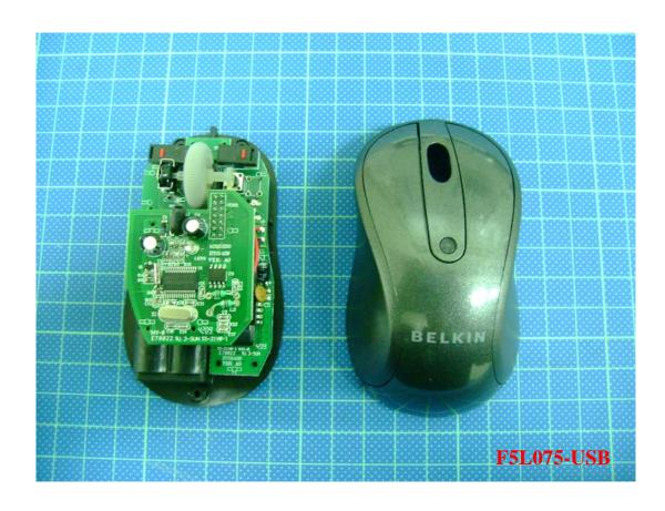
Photo 2: Internal photo of EUT with PCB Printed antenna
