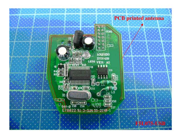
**Photo 3: Internal photo of EUT with PCB Printed antenna**
