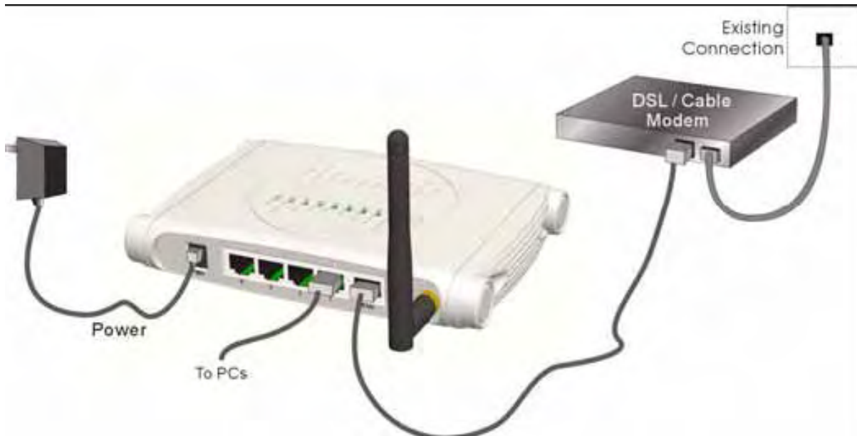
Figure 2-3 Setup of LAN and WAN connections for this product.
