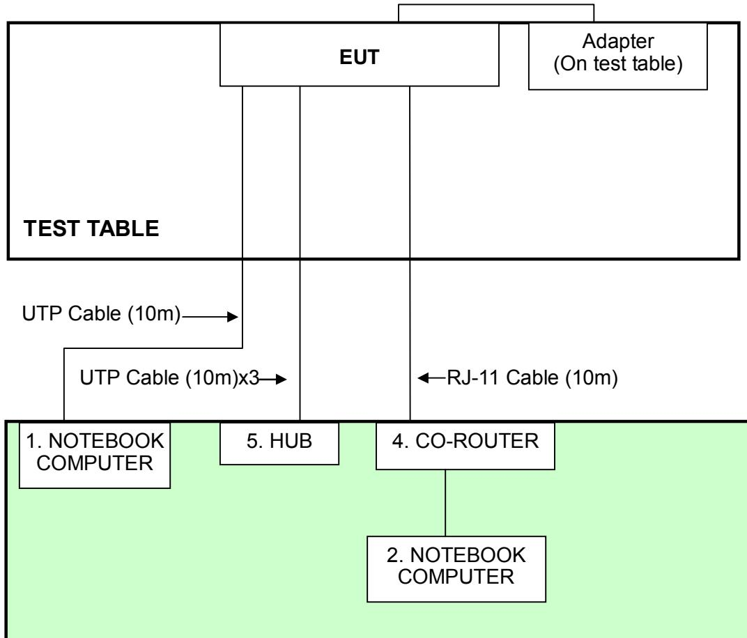
**NOTE:** 1. Support units 1-2, 4-5 were kept in the control room during the test.
