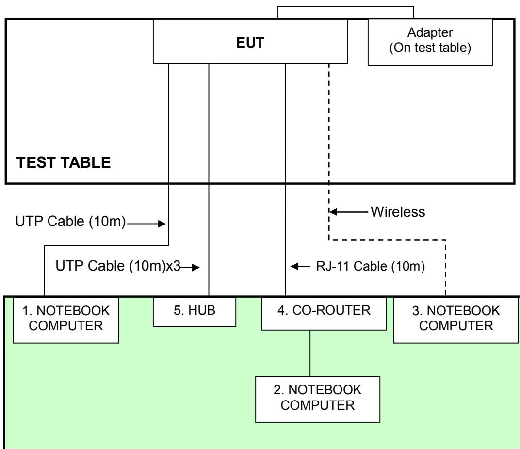
**NOTE:** 1. Support units 1-5 were kept in the control room during the test.
