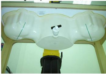
Fig. 5.4 Bottom View of Twin Phantom
