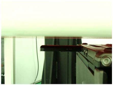
USB Configuration 1 for Back Off SAR (DUT Horizontal Up with Phantom 15 mm Gap)
