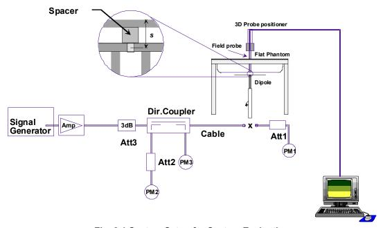
Fig. 8.1 System Setup for System Evaluation
