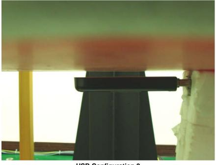
USB Configuration 2 (DUT Horizontal Down with Phantom 5 mm Gap)
