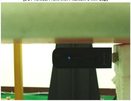
USB Configuration 4 (DUT Vertical Back with Phantom 5 mm Gap)
