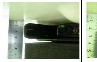
C: NOTEBOOK PP01LD: NOTEBOOK n6000The right edge of the EUT face to the phantom<br/>with 5mm-separation distance.The left edge of the EUT face to the phantom<br/>with 5mm-separation distance.
