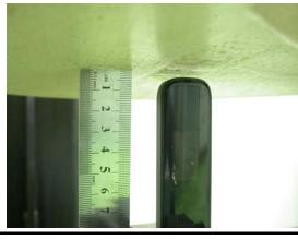
E: NOTEBOOK n6000 The tip of the EUT face to the phantom with 5mm-separation distance.
