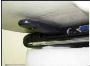
The bottom of the EUT face to the phantom with 7mm-separation distance.
