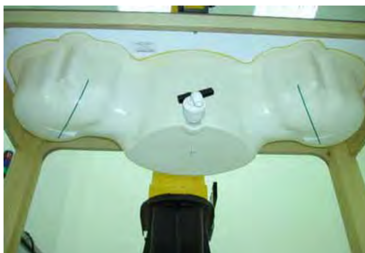
Fig. 5.4 Bottom view of twin phantom
