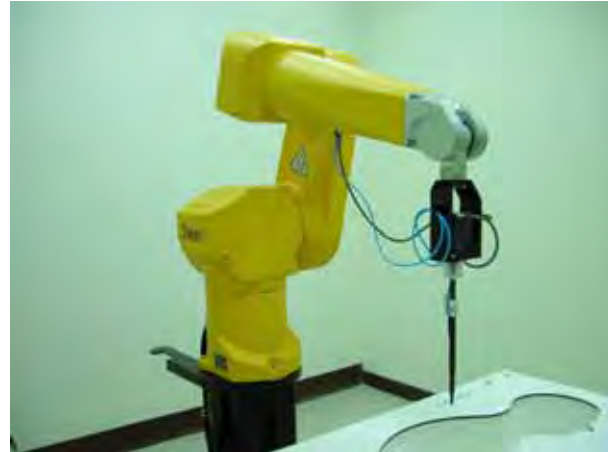
Fig. 5.2 Probe setup on robot
