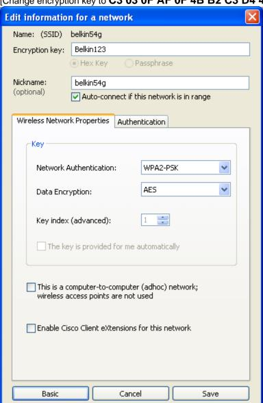
**3.** Click "Save" to finish. Encryption in the wireless router (or access point) is now set. Each of the computers on your wireless network will now need to be configured with the same security settings.
