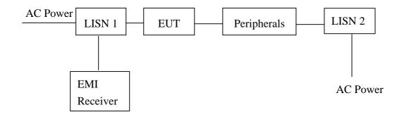
The EUT are connected to the main power through a line impedance stabilization network (LISN). This provides a 50 ohm/50uH coupling impedance for the measuring equipment. The peripheral devices are also connected to the main power through a LISN that provides a 500hm/50uH coupling impedance with 500hm termination.
