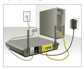
2. After connecting the power adapter and the power source is turned on, the Router's power icon ⊕ on the front panel should be on. It might take a few minutes for the Router to fully start up.
