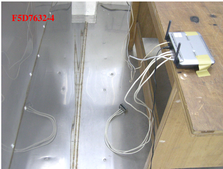
Photo 2: Conducted Emission Test Set-up
