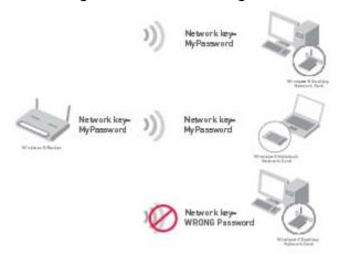
The Wireless G Desktop Network Card cannot access the network because it is using a different Network key than the Network key that is configured on the Wireless G Router.
