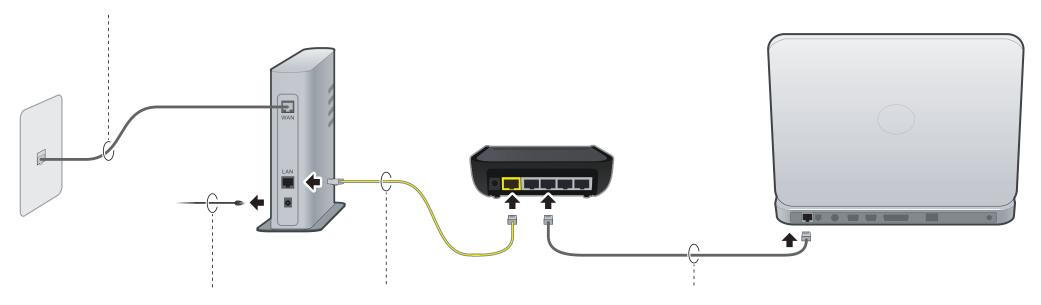
[2] Remove the power cord from your DSL or cable modem.
