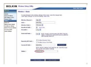
The example below illustrates using Repeater mode to extend the range of your wireless network. In this example, the WURE is set up to connect to the wireless router located in another area.
