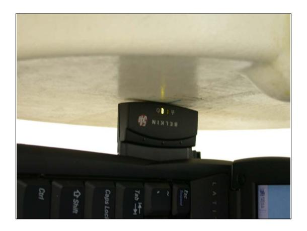
**EUT** to the phantom distance 0mm
