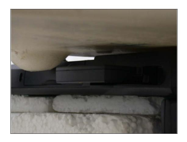
**EUT** to the phantom distance 11mm
