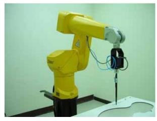
Fig. 5.2 Probe setup on robot
