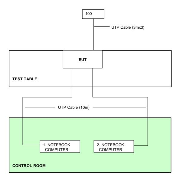
**NOTE:** 1. Support units 1&2 were kept in the control room during the test.
