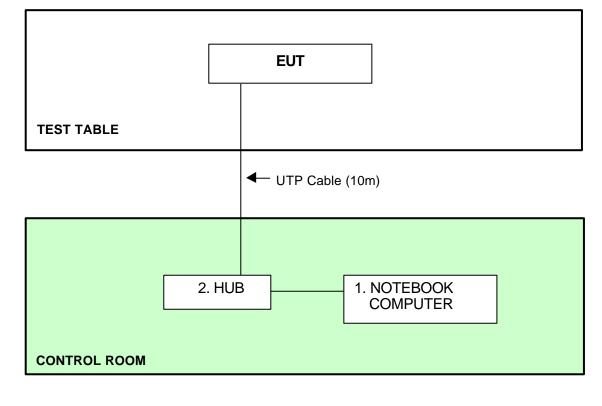
**NOTE:** 1. Support units 1&2 were kept in the control room during the test.
