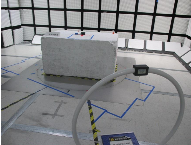
RADIATED EMISSIONS BELOW 30MHz (Front – 10W Load without Airgap)
