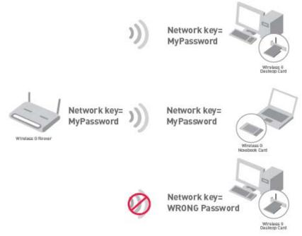
The network adapter cannot access the network because it uses a different network key than the one configured on the wireless router.
