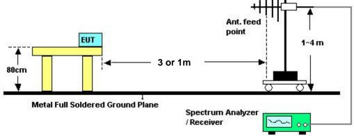
Above 10 GHz shall be extrapolated to the specified distance using an extrapolation factor of 20 dB/decade form 3m to 1m.
