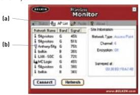
3. Double-click on the network to which you want to connect. A blue circle (b) should appear around the network icon next to the name of the network you selected. This means you are connected to the network. If the network is using encryption security, you will be prompted to make a profile for that network in order to connect. See the section of this User Manual called "Profile Tab: Creating a Profile" on page 16 for information.
