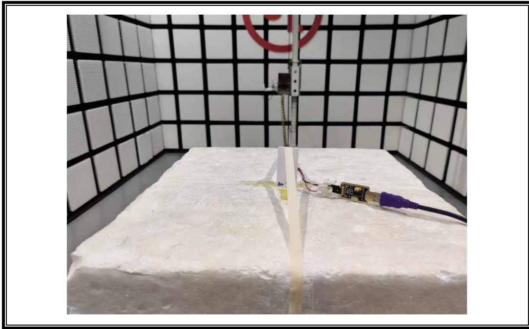
RADIATED RF MEASUREMENT SETUP (Above 1G – X axis)
