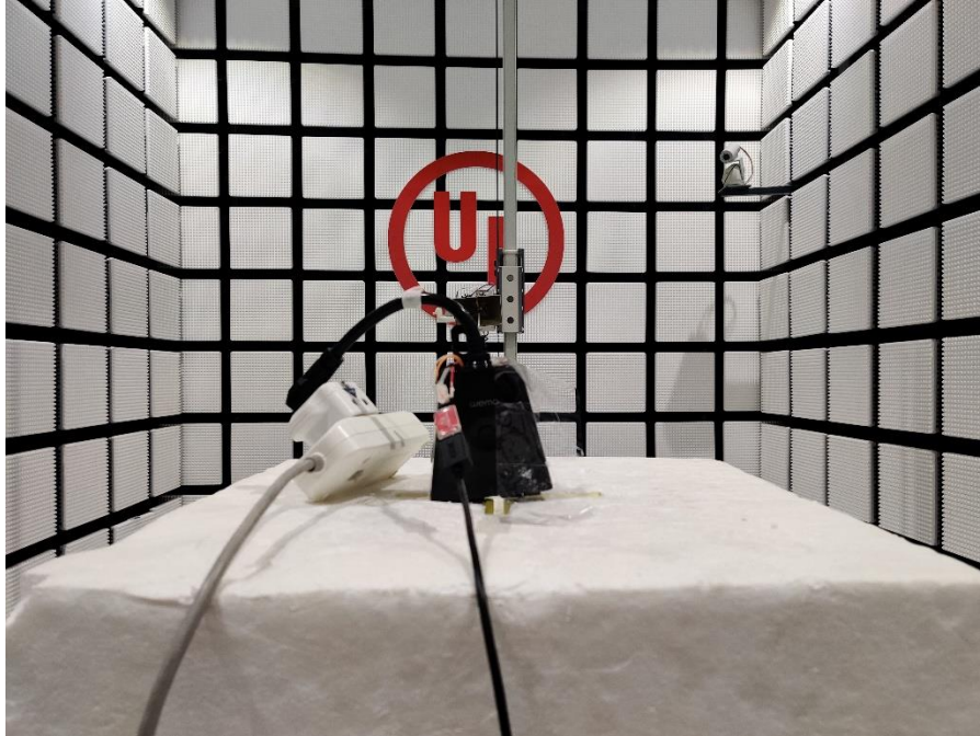
RADIATED RF MEASUREMENT SETUP (30MHz~1GHz)
