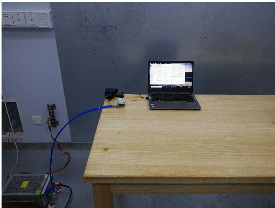
POWERLINE CONDUCTED EMISSIONS MEASUREMENT SETUP
