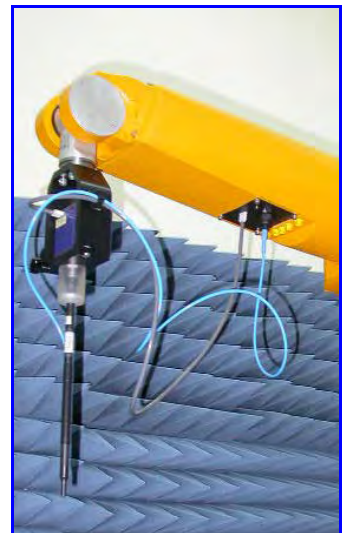
Figure 12. Probe setup on robot
