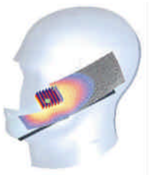
Figure 7.1 Sample SAR Area Scan
