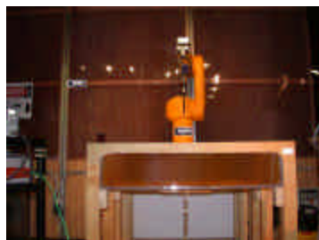
Figure 12.1 Dipole Validation Test Setup
