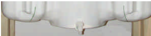
Figure 7.2 SAM Twin Phantom shell
