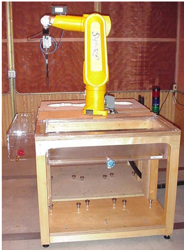
DASY4 SAR Measurement System with validation phantom
