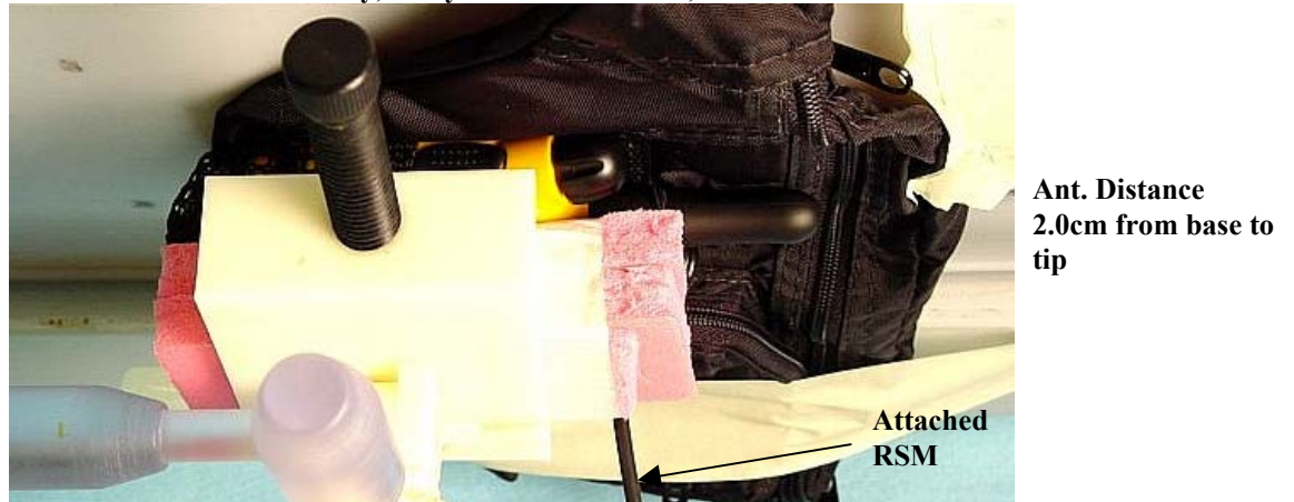
Figure 4. Assessment @ the Abdomen; DUT w/ AA Alkaline battery, carry case model 50982, and RSM model NTN8867A
