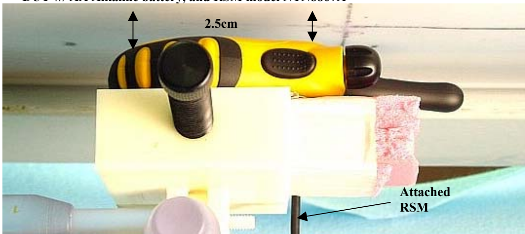
Figure 6. Assessment @ the Abdomen; DUT Back 2.5cm separation from phantom DUT w/ AA Alkaline battery, and RSM model NTN8867A
