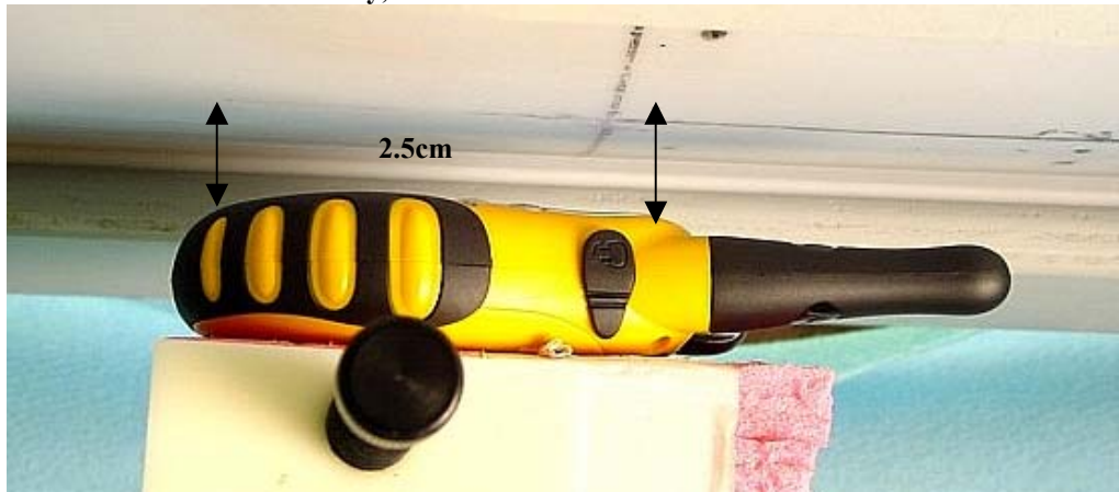
Figure 8. Assessment @ the Face; DUT front 2.5cm separation from phantom DUT w/ AA Alkaline battery, and RSM model NTN8867A
