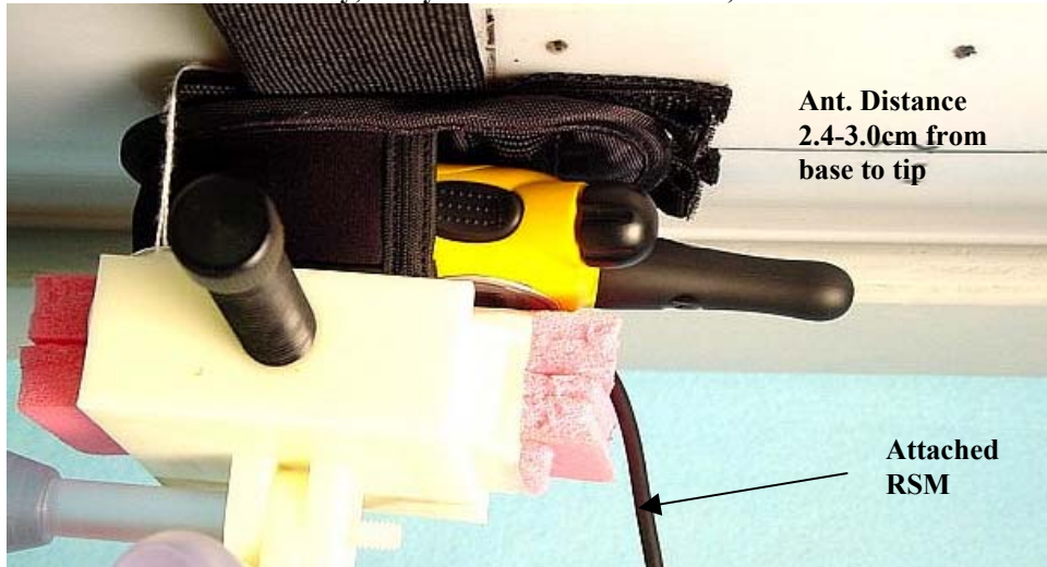
Figure 3. Assessment @ the Abdomen; DUT w/ AA Alkaline battery, carry case model NTN9399B, and RSM model NTN8867A
