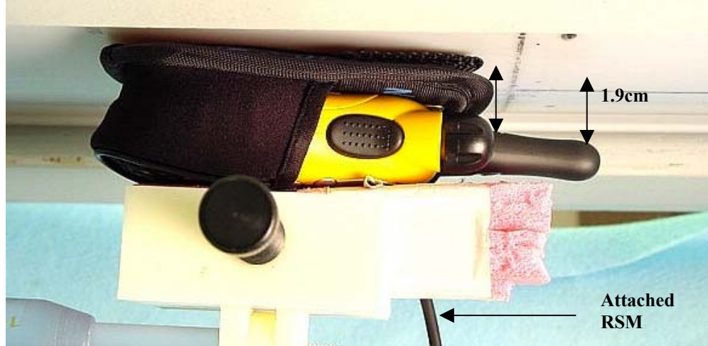
Figure 1. Assessment @ the Abdomen; DUT w/ AA Alkaline battery, belt clip model NTN9153A, and RSM model NTN8867A (Note: All other offered audio accessories were assessed while attached to the DUT in this position)
