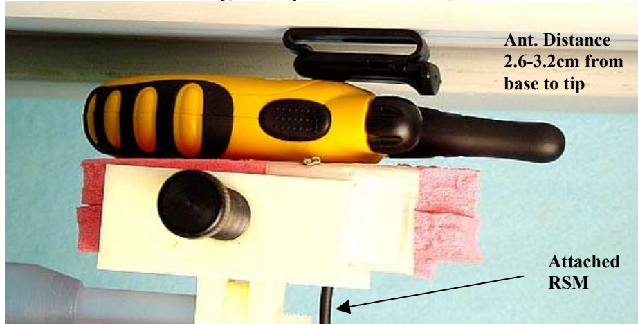
Figure 2. Assessment @ the Abdomen; DUT w/ AA Alkaline battery, belt clip model NTN9392B, and RSM model NTN8867A
