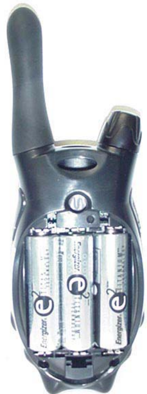
DUT with Energizer E-Squared AA Alkaline Batteries
