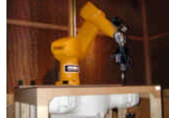
Figure 6.1 DASY4 Test System
