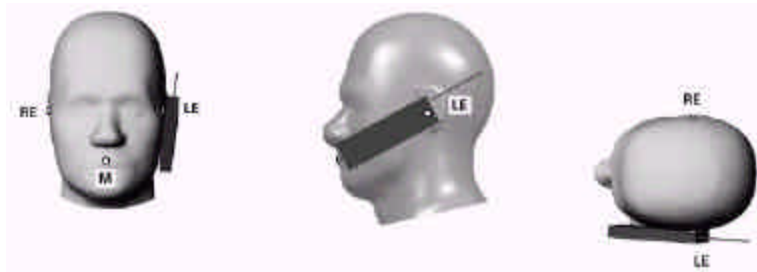
Figure 9.1 Front, Side and Top View of Cheek/Touch Position
