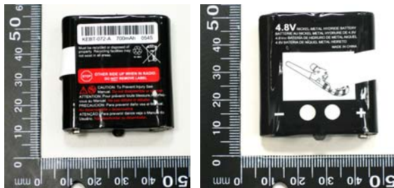
Ni-MH Battery ( 4.8V 700mAh )
