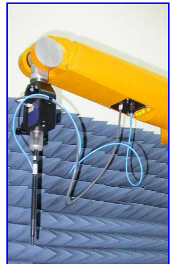
Figure 10. Probe setup on robot
