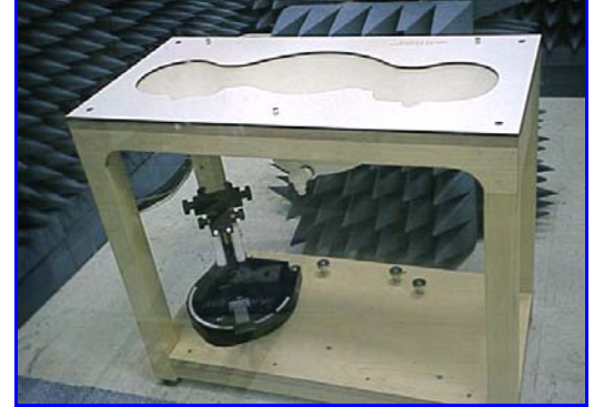
Figure 12. SAM Twin Phantom
