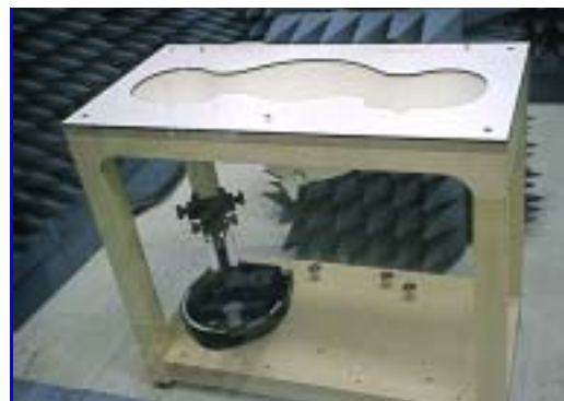
Figure 8. SAM Twin Phantom
